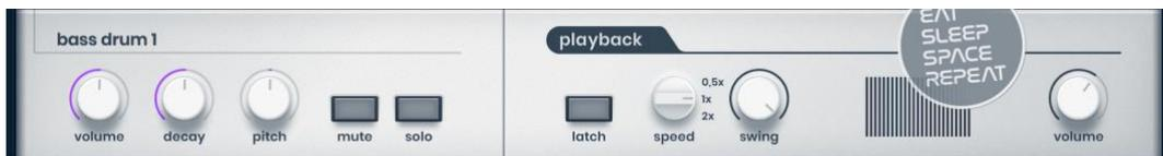
With Latch on, Beatmaker EDEN will keep playing after keys are released, until either Latch is switched off or the Sto key (B4) is pressed.
